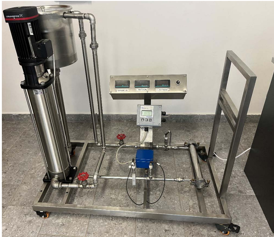
Figure 2 Additional membrane filtration unit in the TFNS laboratories
