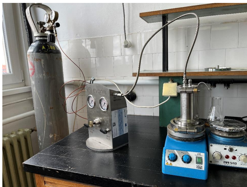
Figure 4. METcell® dead-end filtration unit installed at the TFNS laboratory labeled with TwINSol-CECs sticker
